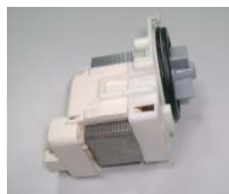
Pompe de vidange 30W – 17-21L/sec – 143ohm ±7% - Protection thermique 120C°
